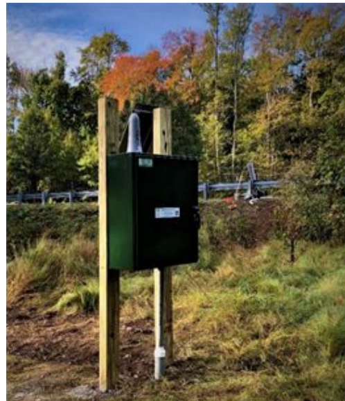
Figure 1. Photograph of a streamgage similar to what will be installed on Long Branch.
