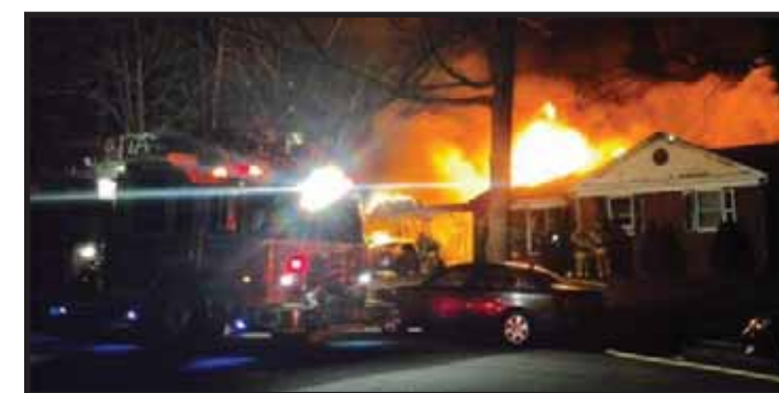
This accidental house fire in the Oakton area on March 30, 2016, was started by rags that were soaked with linseed oil that were left in a pile outside of the home. The rags spontaneously combusted and caused the fire to spread to the home. The home sustained approximately $652,500 in damages. (Top two and bottom left photos provided by Dereck Welsh, Northern Virginia Fire Buffs. Bottom right photo by Battalion Chief Willie Bailey.)
