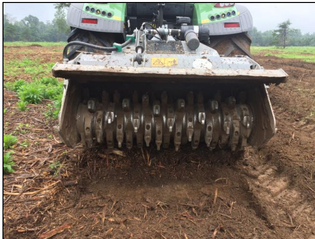
Management Unit 24 – Summer 2017: FAE forestry tiller incorporating woody debris
