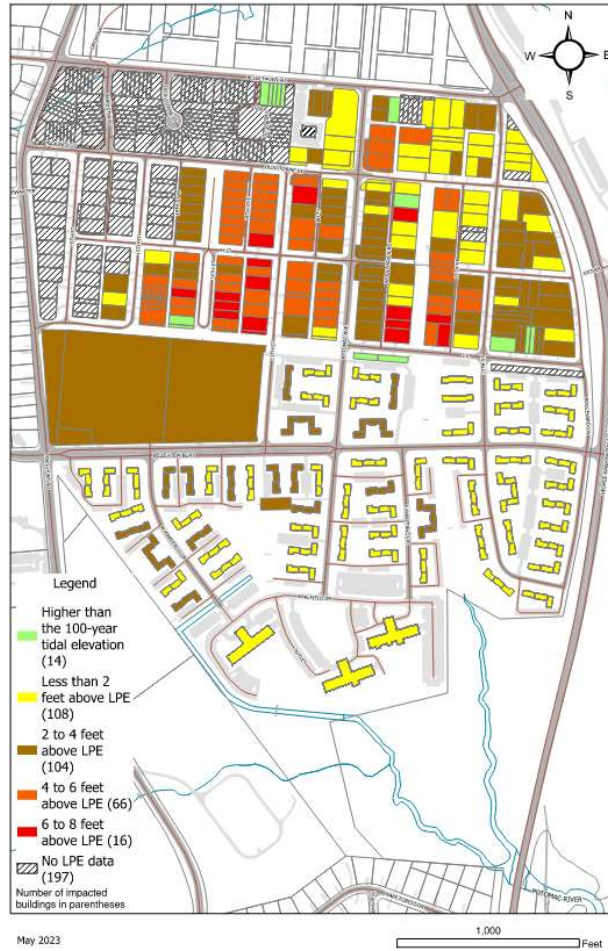
Depth of flooding above building Lowest Point of Entry (LPE) for 100-year tidal elevation at Belle Haven
