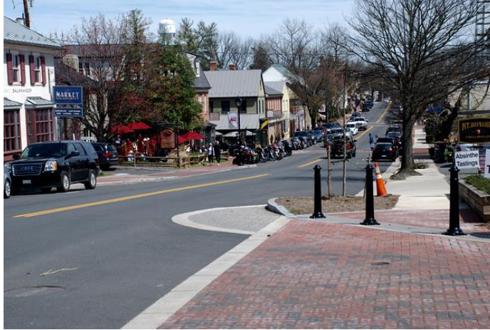
Figure 7 Example of reduced radii installed by VDOT along Route 50 in Middleburg with a mountable apron for truck and trailer
