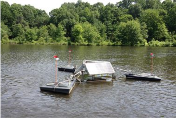
Solar powered water circulator
