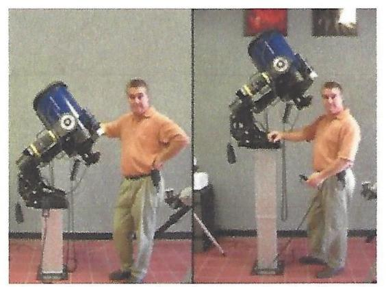
Pier Tech Inc photo demonstrating the motorized adjustable height pier.
