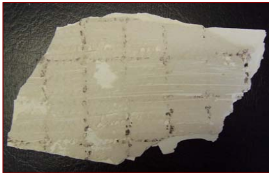
Image 3.57: Wallpaper Design Adhering to Back of Paint Sample
