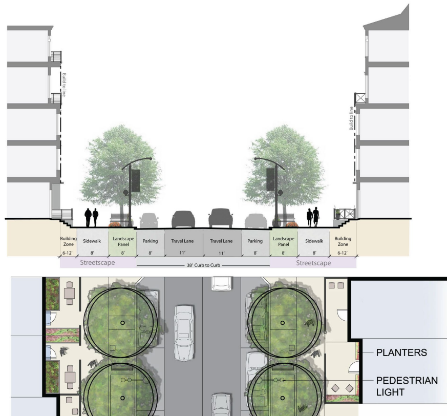
Figure 38 – Local Street Cross-section
