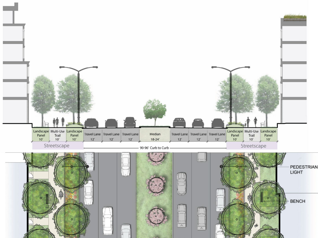
Figure 34 – Multimodal Through Corridor Cross-section
