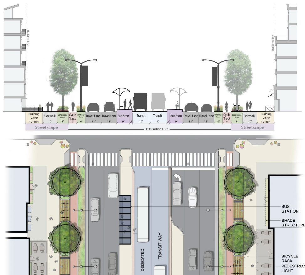
Figure 35 – Transit Boulevard Median Running Cross-section
