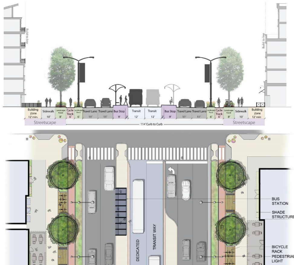
Figure 34 – Transit Boulevard Median Running Cross-section
