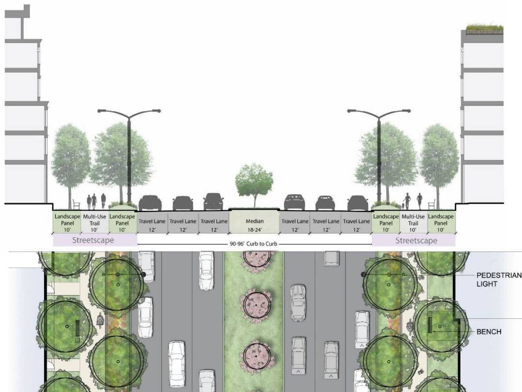
Figure 33 – Multimodal Through Corridor Cross-section
