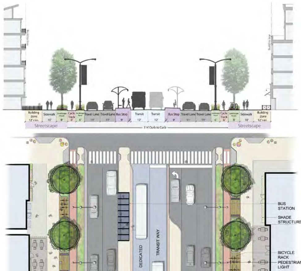
Figure 35 – Transit Boulevard Median Running Cross-section
