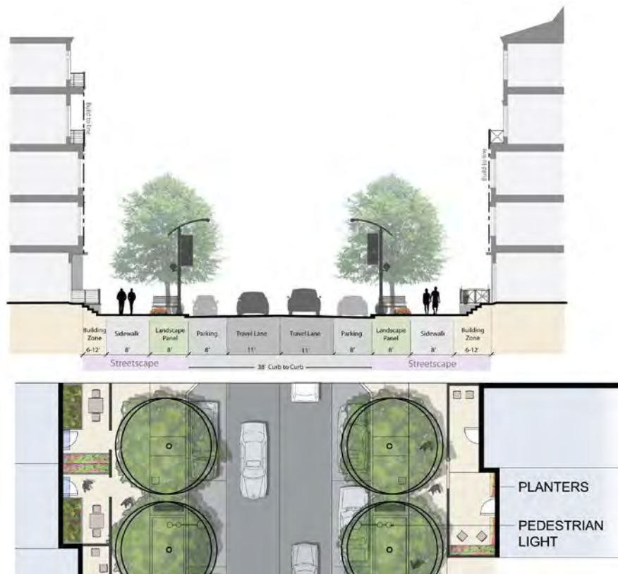
Figure 38 – Local Street Cross-section
