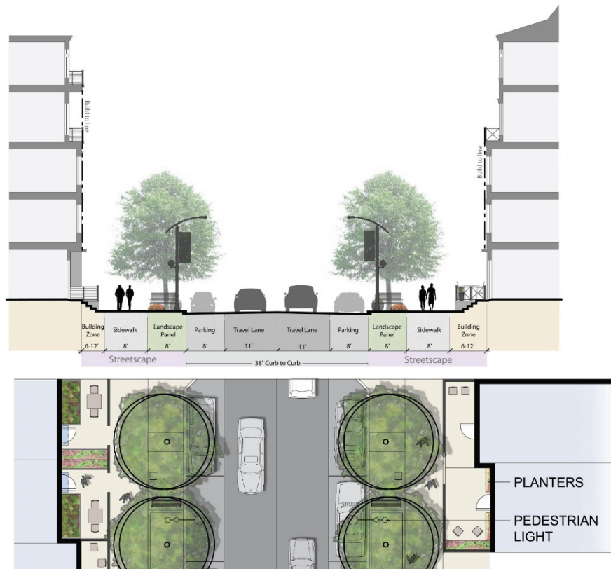
Figure 38 – Local Street Cross-section
