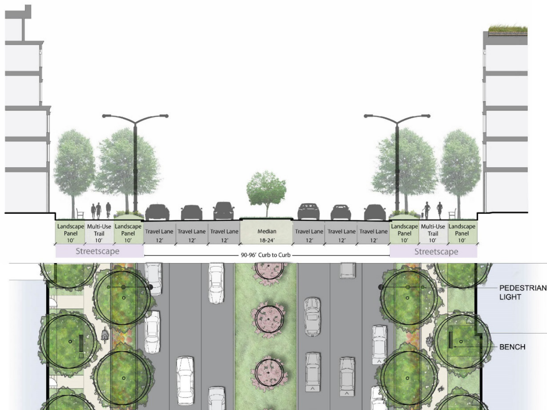
Figure 34 – Multimodal Through Corridor Cross-section
