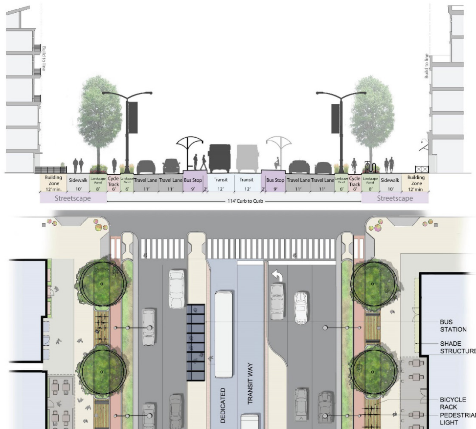
Figure 35 – Transit Boulevard Median Running Cross-section
