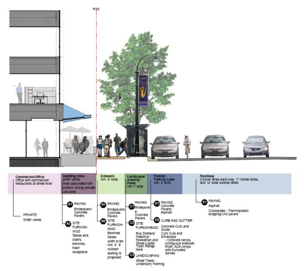
Figure 18: Collector Street Half-section
