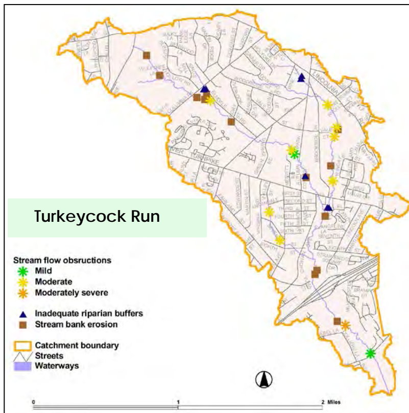
Figure 4-24. Location of major problems in Turkeycock Run subwatershed as indicated by SPA data
