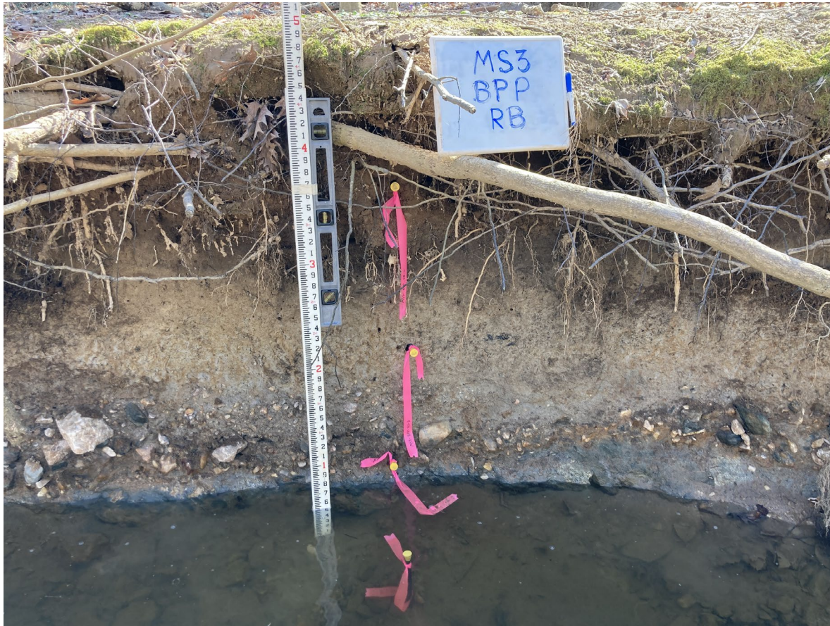
Bank Pin Measurement in March 2022 (initial installation)
