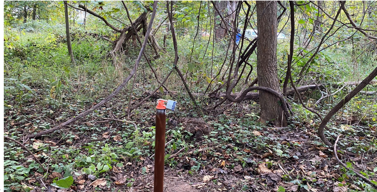
Groundwater logger installation.
