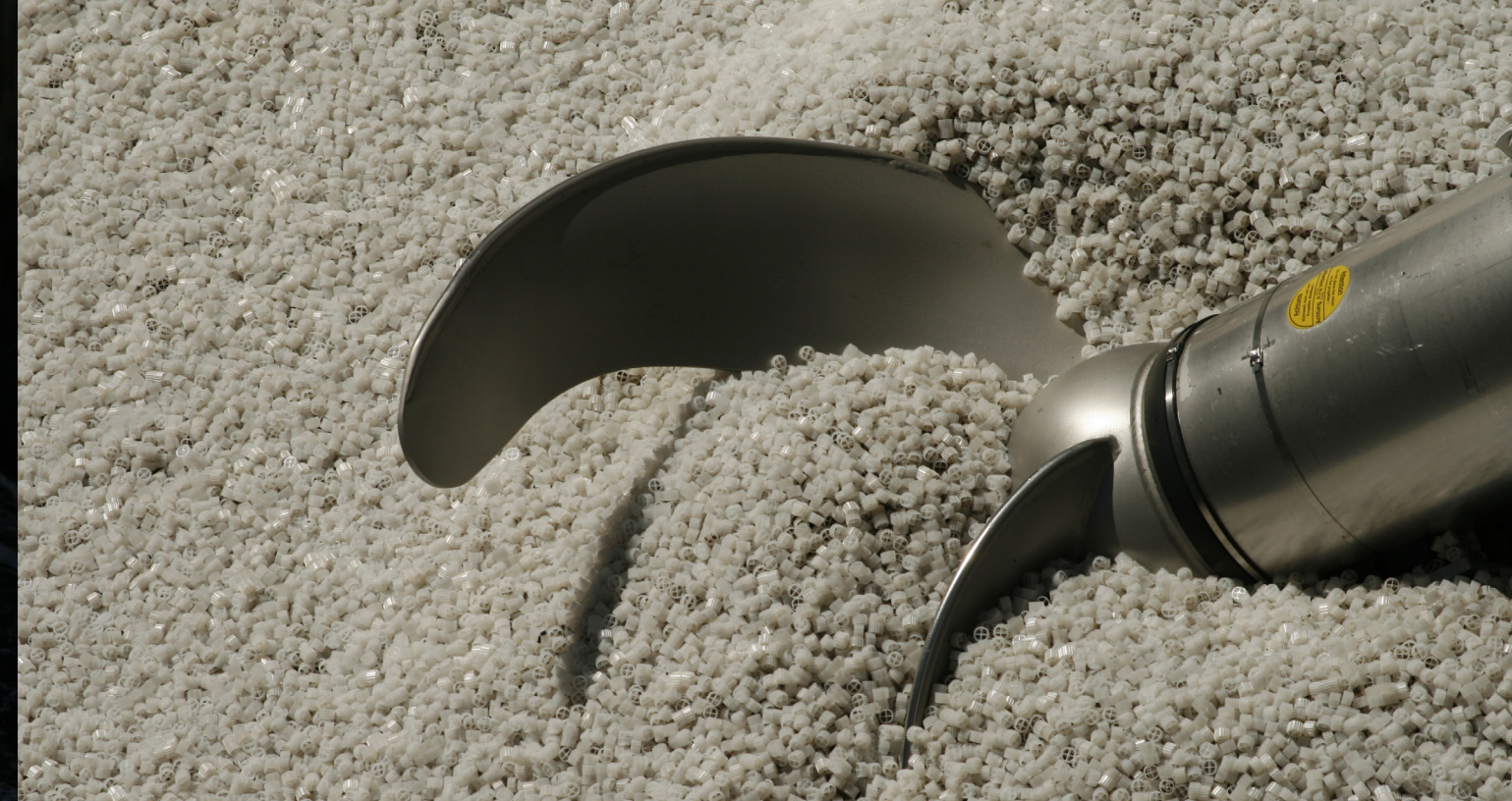
Plastic growth media for nitrogen removal.
