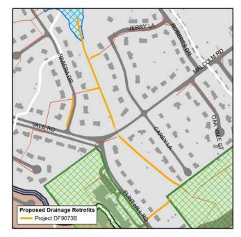
systems with more natural drainage. The upstream flume would be removed and replaced with a dry swale. The lower reach would be reconstructed as a natural stream channel with step pools to reduce flow velocity. Riparian buffer should be reestablished where deficient.
