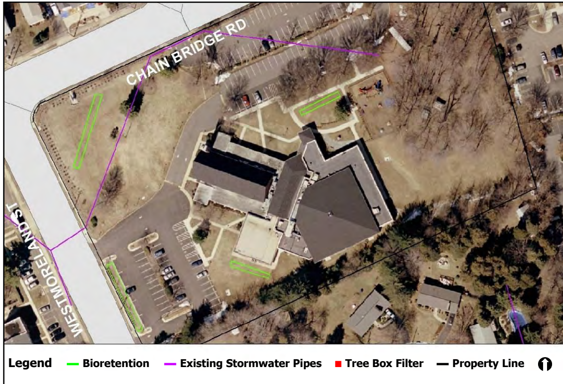
Project Area Map: Conceptual plan of 1545 Chain Bridge Road showing potential locations of LID measures
