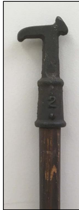
Pole Hook used to Open Windows in Clerk's 2nd Office and Clerk's Addition, c. 1910 - 1935
