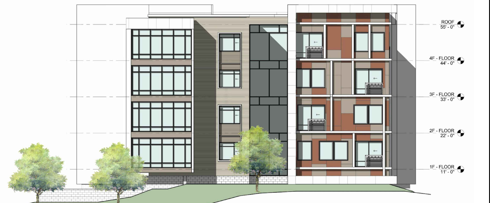
4 BUILDING 1B - SOUTH ELEVATION
