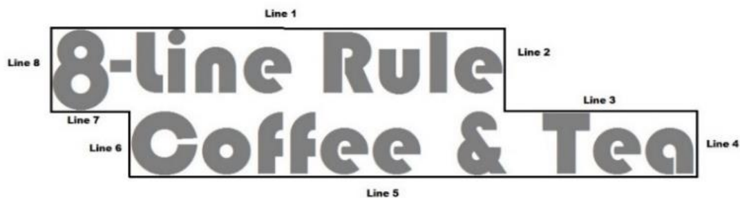
Figure 7100.2: Measuring Building-Mounted Sign Area
