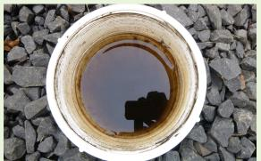
Photo 4 - Standing water observed inside observation well for more than 48 hours.
