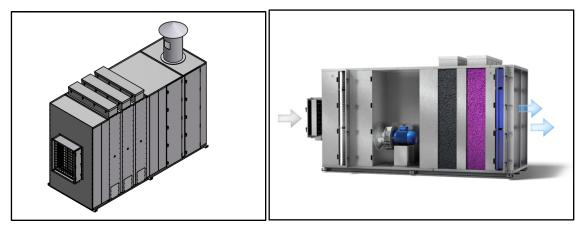
Carbon adsorption is most cost-effective for  $H_2S$  concentrations of less than 10 ppm  $H_2S$ , as concentrations greater than 10 ppm will accelerate carbon replacement requirements. The estimated carbon media life with <5 ppm  $H_2S$  concentration is 3 years.
