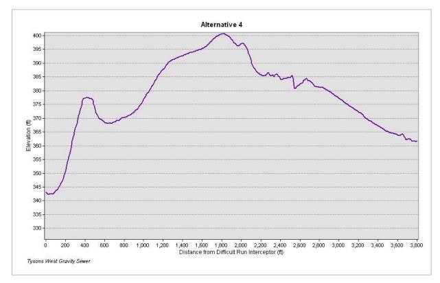
Figure-9: Grade elevation for Alternative-4 route
