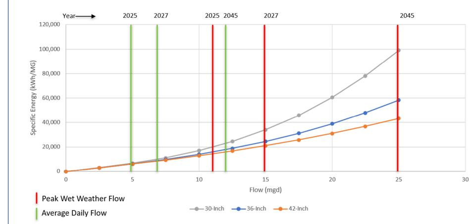
Figure 3-7: Specific energy profile for three different force main diameter alternatives.
