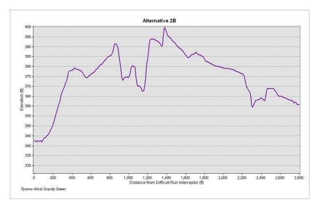
Figure-5: Grade elevation for Alternative-2B route
