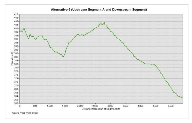
Figure-11: Grade elevation for Alternative-5 route
