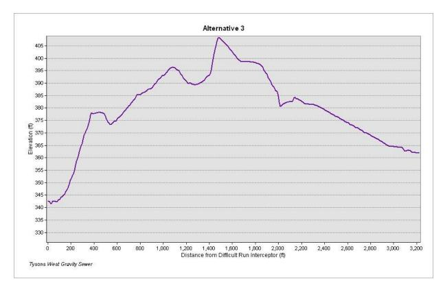
Figure-7: Grade elevation for Alternative-3 route
