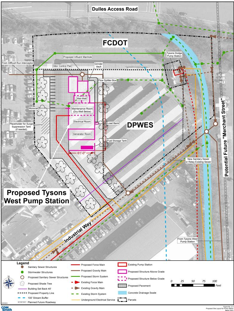
Figure No. 2-Proposed Site Layout for Pump Station
