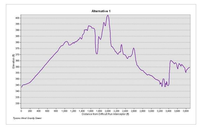
Figure-2: Grade elevation for Alternative-1 route
