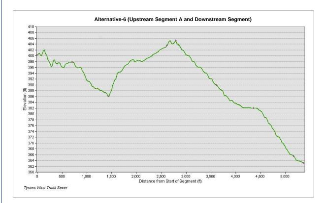
Figure-14: Grade elevation for Alternative-6 route Upstream Segment A and Downstream Segment
