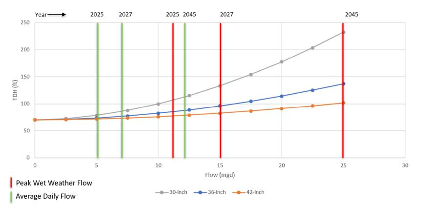
Figure 3-6: Total dynamic head profile for three different force main diameter alternatives.
