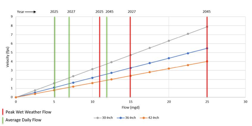
Figure 3-4: Velocity profile for three different force main diameter alternatives.
