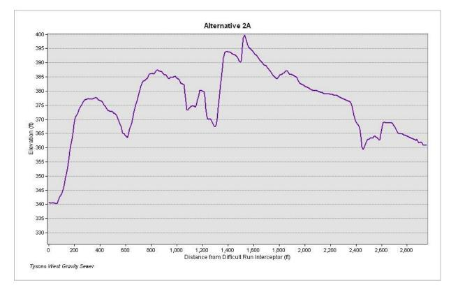
Figure-4: Grade elevation for Alternative-2A route
