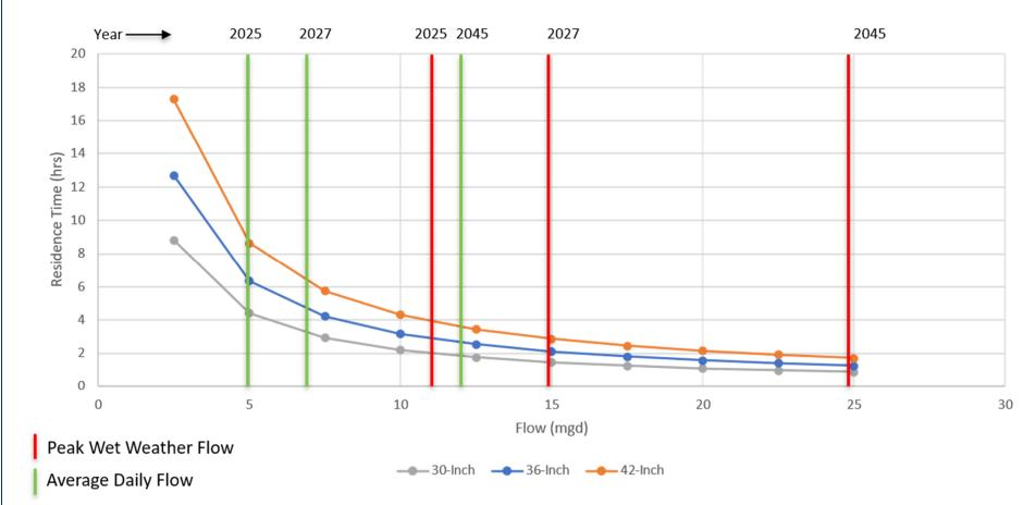
Figure 3-5: Residence time profile for three different force main diameter alternatives.
