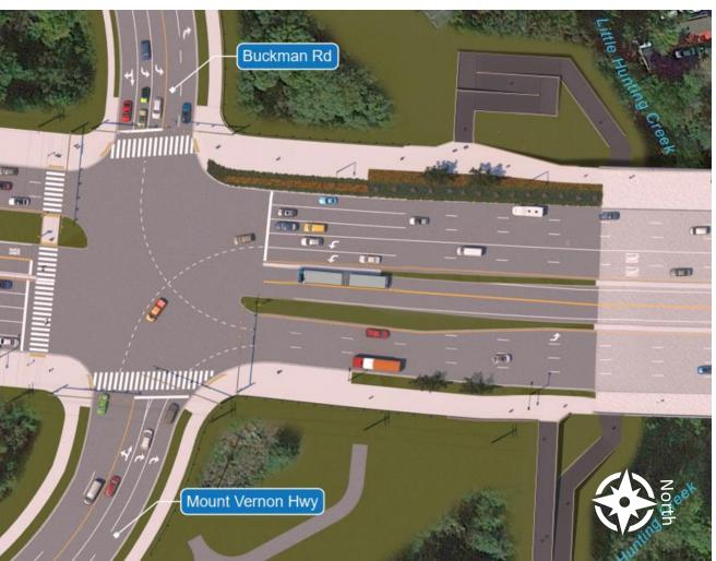
The rendering depicts the intersection in the hypothetical situation in which the exclusive SB right-turn lane is removed after construction of the project based on an evaluation of land development & other conditions.
