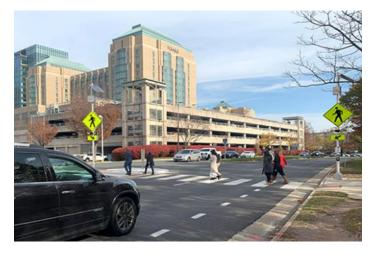
Rectangular Rapid Flash Beacon (RRFB) are bright flashing lights that are activated by pushing a button. The lights warn drivers that a person is crossing the road. Pedestrians still have to wait for a safe gap in traffic before crossing.
