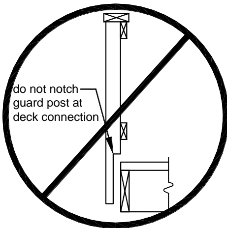
FIGURE 29: NOTCHING AT GUARD POSTS
