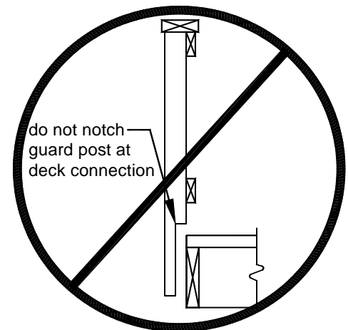
FIGURE 27: PROHIBITED NOTCHING AT GUARD POSTS
