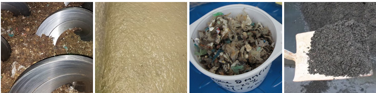
Figure 7: Input and Products from the Organics Polishing System (Left to Right) - Infeed from OREX™, Polished Wet Fraction, Light Rejects, Heavy Rejects
