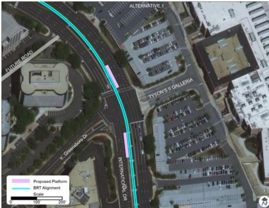
Figure 8-7 | Greensboro Road Station Location and Platform Configuration
