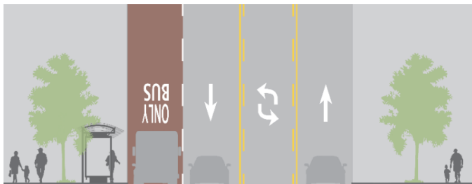
Figure 6-25 | Alternative 6 Cross-section of Boone Boulevard from Spring Hill Road to Chain Bridge Road
