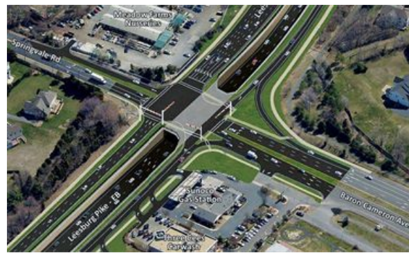
EXAMPLE OF AN ECHELON INTERCHANGE Source: VDOT
