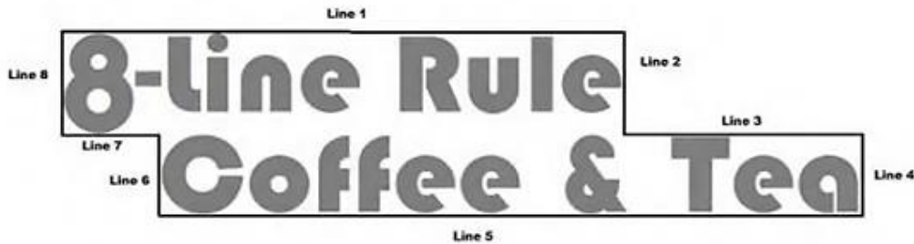
Figure 7100.2: Measuring Building-Mounted Sign Area
