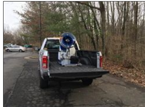
Figure 23: Ultra-low volume sprayer mounted in the back of a pick-up truck.
