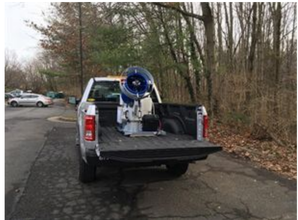
Figure 14: Ultra-low volume sprayer mounted in the back of a pick-up truck.
