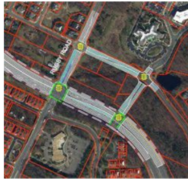
RUGBY ROAD QUADRANT INTERSECTION
