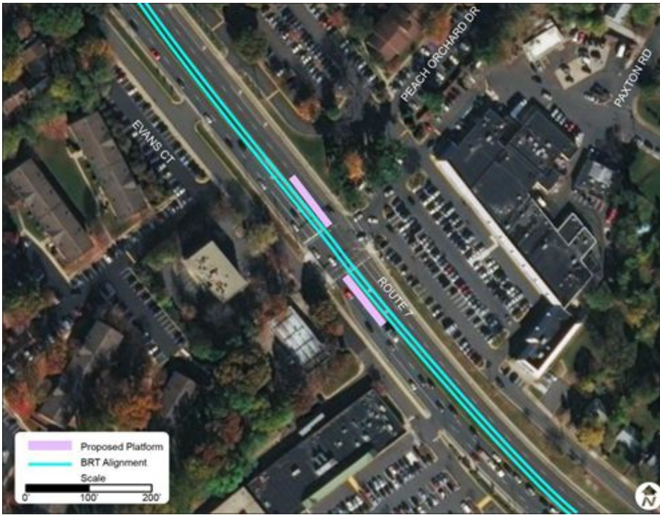
Figure 8-17 | Patterson Road Station Location and Platform Configuration
