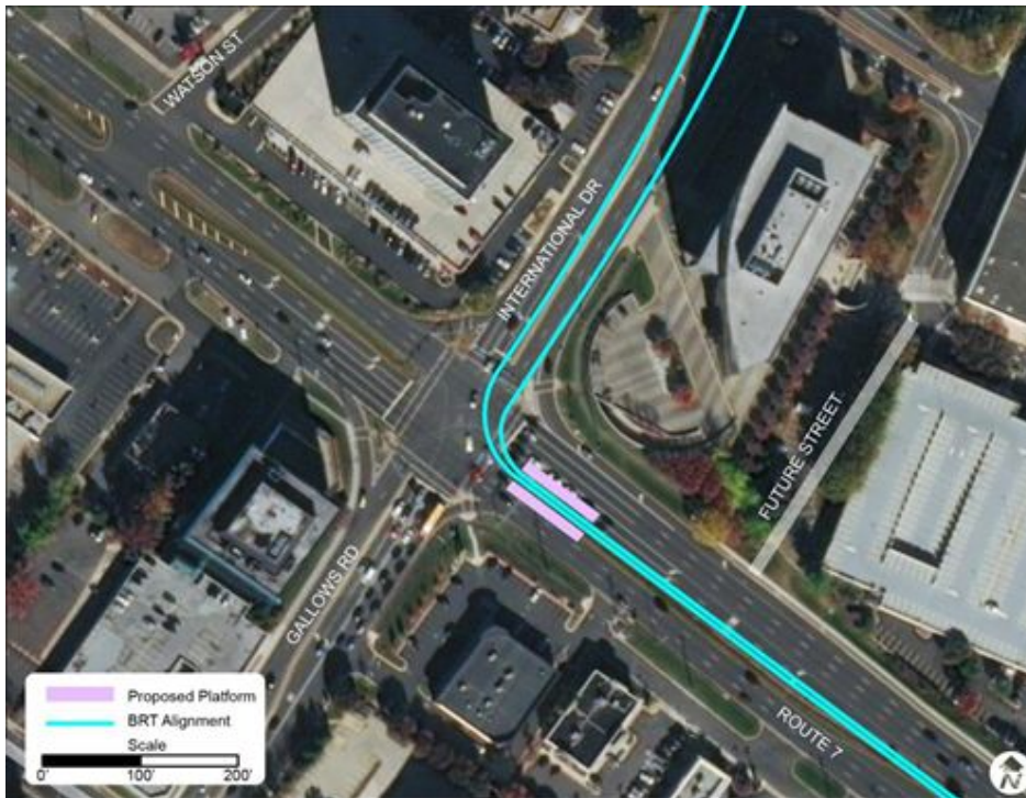
Figure 8-13 | International Drive Station Location and Platform Configuration
