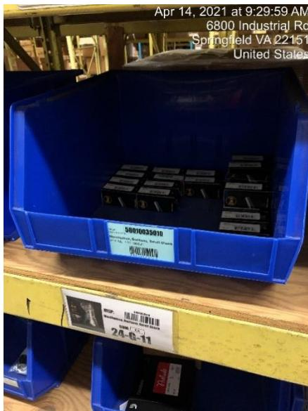
Figure 2-2. Bulk items are removed from initial packaging and stored in individual organized containers.
