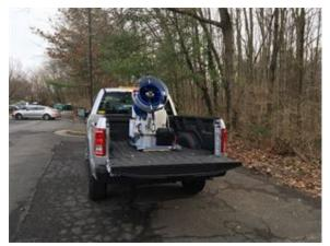
*Figure 12: Ultra-low volume sprayer mounted in the back of a pick-up truck.*
