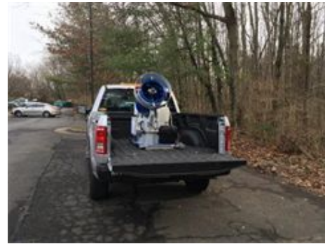
Figure 17: Ultra-low volume sprayer mounted in the back of a pick-up truck.
