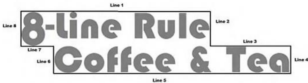
Figure 7100.2: Measuring Building-Mounted Sign Area
