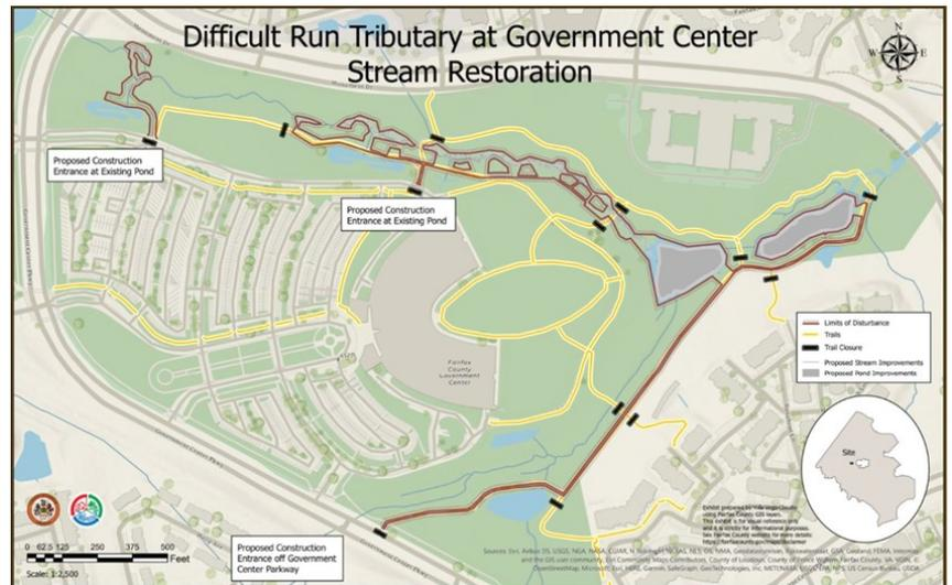
The project will involve grading, excavation and filling of soil, stream alignment, installation of in-stream and log structures, riparian corridor improvement, native species landscaping, and trail restoration. Before contractors dredge the ponds, County staff will relocate fish and other aquatic life to the Herrity Building Pond. Upon completion, SWPD will restock the two Government Center ponds.
