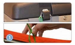
Verify the green seal number securing the black DS200 lid matches the **Machine Certification**Form. Once verified, cut the seal and place it inside of the #7 Orange Pouch.
