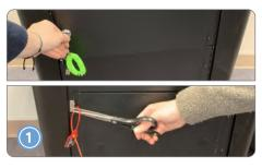
Cut the zip-tie seal on the Ballot Compartment. Unlock and open the Auxiliary and Ballot Compartments. Verify that they are empty, then re-lock them. (Ensure the metal bar is in the up and locked position.) Seal the Ballot Compartment with a new barcoded zip-tie seal.
