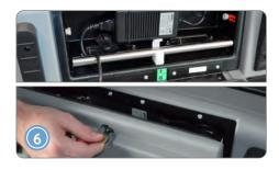
Unplug the power cord, then re-wrap the cord and place it back inside the Power Cord Compartment. Close and lock the compartment.
