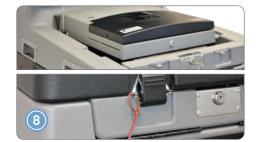
Close and re-lock the DS200 screen, followed by the black machine lid. After re-hooking the lid latches, secure the black machine lid with a red zip-tie seal, then record the seal number on the **Machine Certification Form.** Repeat steps 1-8 for each DS200 used.
