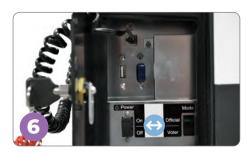
Verify the mode switch is set to **Voter**, then flip the power switch to **On**. The ExpressVote will take about three minutes to fully power on.
