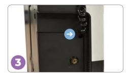
Position the keypad cord through the opening at the top of the Access Door. Close and re-lock the door.
