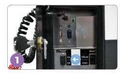
Open the Access Door with the black barrel key, and flip the power switch to **Off**. Do not detach the keypad. The ExpressVote will take about three minutes to power down.
