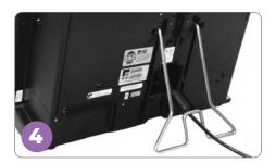
Lift out and extend the metal prop bar on the back of the ExpressVote. Position the device so that it is stable and rests upright at a slight angle.
