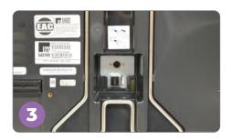
Put together the power cord and plug into a surge protector. Plug the surge protector into an outlet. Plug the other end of power cord into the power connection port on back of the ExpressVote. Insert the cord until you hear a click to ensure cord is secure.
