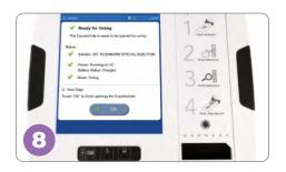
On the screen, verify that the precinct number and name are correct. Verify that the unit is receiving power by looking for the green light below the screen. Tap **OK**. Close and re-lock the Access Door, ensuring that the keypad cord threads through the opening at the top of the access door.
