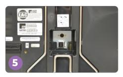
Unplug the power cord from the back of the ExpressVote. Pull the release latch on the cord to remove it. Next, unplug the power cord from the surge protector, and unplug the surge protector from the wall outlet.
