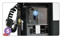
Open the Access Door on left side of ExpressVote with the black barrel key. Verify that the keypad is plugged into the keypad port. Place the headphones and keypad on the table so they are accessible for voters. (Keep headphones unplugged unless a voter is using them.)
