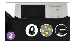
Remove the ExpressVote, headphones, and keypad from main compartment of the black padded carrying case. Remove the power cord from the side compartment of case, then return the black padded case to gray supply cart.
