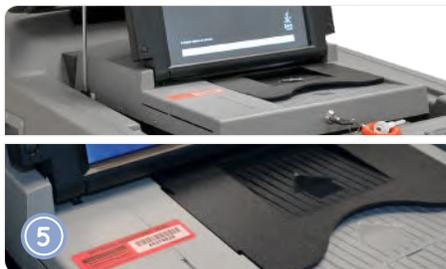
Unlock and open the Ballot Box lid, followed by the DS200. Lift and raise the DS200 screen to power on the scanner, then verify the red barcoded seal matches the Machine Certification Form.
