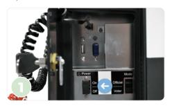
**NEW:** Remove memory device from all ExpressVote machines and place in orange #7 pouch. Position keypad so it threads through circular opening at top of Access Door. Close and relock door.
