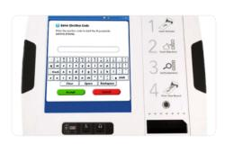
Verify precinct number/name on screen is correct and unit is receiving power. Touch **0k**. Place keypad cord so it threads through circular opening at top of Access Door. Close and relock door.
