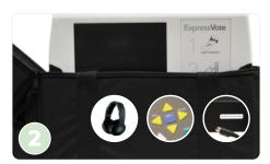
Plug power cord into power strip, then into AC outlet. Plug other end of power cord into power connection port on back of ExpressVote. Insert cord until you hear a click to ensure cord is secure.
