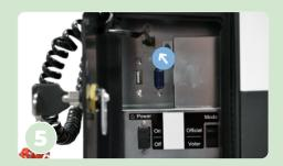
Verify mode switch is set to **Voter**, then flip power switch to **On**. ExpressVote powers on and boots up (device takes approximately three minutes to fully power on).
