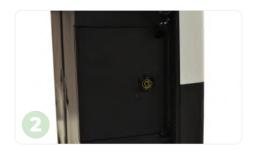
Close metal prop bar on back of ExpressVote and position device so it rests in an upright position on its base.
