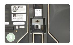
Lift out and extend the metal prop bar on back of ExpressVote. Position device so that it rests in an upright position at a slight angle.
