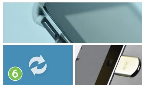
On the Poll Pad, press and hold the **Power** button until the Apple logo appears. After the Poll Pad powers on and the app launches, insert the iSync Drive into the Lightning Connector.
