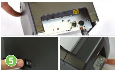
Remove the Printer and its supplies from the Poll Pad Case. Plug the Power Cord into the Adapter, then plug the cord into the Printer. Flip the power switch to **ON**, then press the **Feed** button.
