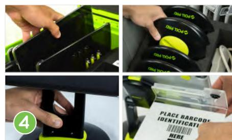
Remove the contents from the Poll Pad Case and Plastic Tote. Assemble each Poll Pad by inserting the Poll Pad Arm into the Base and attaching the Photo ID Holder to the back of the Poll Pad.
