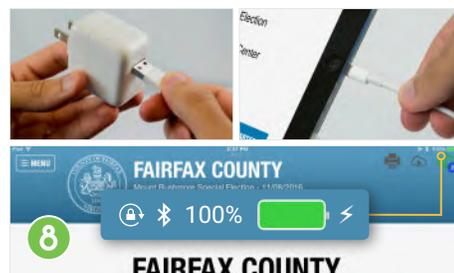
Remove the Power Cube and Cable from the Poll Pad Case. Assemble the cube, then plug the cable into the Lightning Connector. Verify the battery indicator turns green and a **Charge** icon appears.
