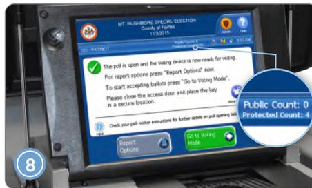
On the screen, verify that the Public Count is zero and the Protected Count matches the **Machine Certification Form**.
