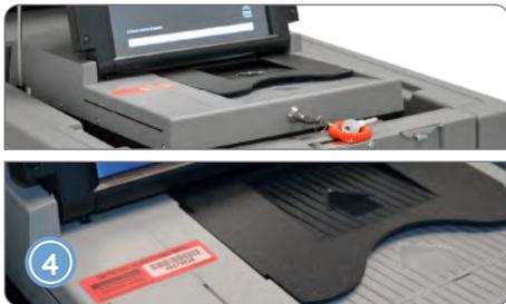
Unlock and open the black DS200 lid. Next, unlock and raise the screen to power on the scanner. Verify the red barcoded sticker seal matches the **Machine Certification Form**.
