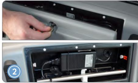
Unlock and open the Power Cord Compartment (back of the machine). Use a surge protector to connect the power cord to an outlet. Verify the metal bar is firmly in the down position and is secured by the white plastic clip. Leave the compartment open for ventilation.
