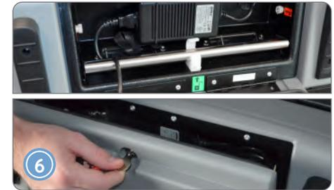
Unplug the power cord, then re-wrap the cord and place it back inside the Power Cord Compartment. Close and lock the compartment.
