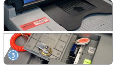
Remove the red barcoded sticker seal and affix it to the **Machine Certification Form**. Unlock and open the Access Door, then press and hold down the physical **Close Poll** button for 3 seconds.
