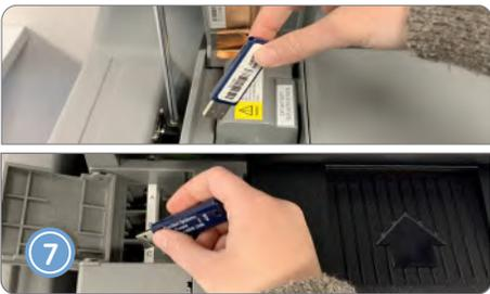
Remove the memory sticks from the Battery Compartment (behind screen) and the Printer Compartment (in front of screen). Give both (2) to the Chief, then close and re-lock both Access Doors. Remove all memory sticks, even if a DS200 was not used.
