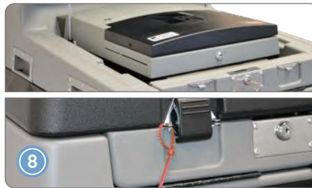
Close and re-lock the DS200 screen, followed by the black machine lid. After re-hooking the lid latches, secure the black machine lid with a red zip-tie seal, then record the seal number on the **Machine Certification Form**. Repeat steps 1-8 for each DS200 used.
