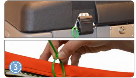
Verify the green voting seal number securing the black DS200 lid matches the **Machine Certification Form**. Once verified, cut the seal and place it inside of the **#7 Orange Pouch**.
