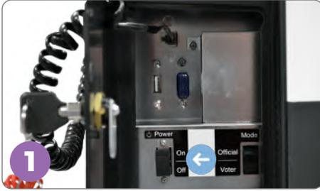
1 Open the Access Door with the black barrel key, and flip the power switch to **Off**. Do not detach the keypad. The ExpressVote will take about three minutes to power down.
