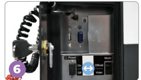
6 Verify the mode switch is set to **Voter**, then flip the power switch to **On**. The ExpressVote will take about three minutes to fully power on.
