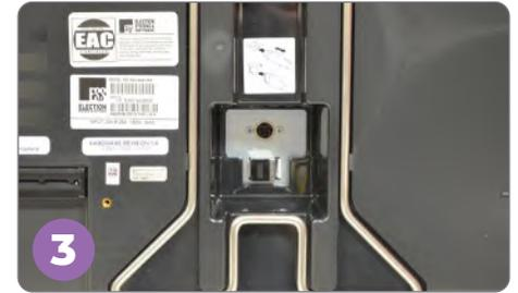
3 Put together the power cord and plug into a surge protector. Plug the surge protector into an outlet. Plug the other end of power cord into the power connection port on back of the ExpressVote. Insert the cord until you hear a click to ensure cord is secure.
