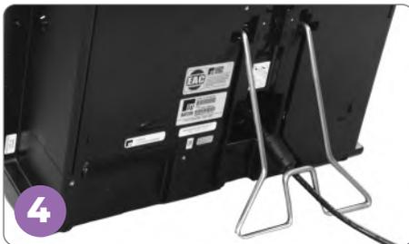
4 Lift out and extend the metal prop bar on the back of the ExpressVote. Position the device so that it is stable and rests upright at a slight angle.
