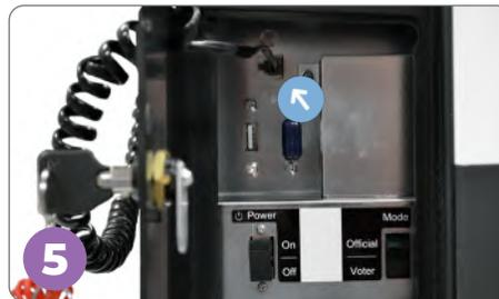
5 Open the Access Door on left side of ExpressVote with the black barrel key. Verify that the keypad is plugged into the keypad port. Place the headphones and keypad on the table so they are accessible for voters. (Keep headphones unplugged unless a voter is using them.)
