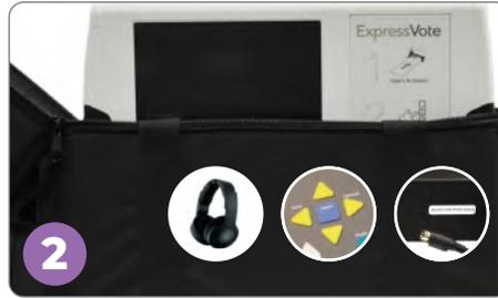
2 Remove the ExpressVote, headphones, and keypad from main compartment of the black padded carrying case. Remove the power cord from the side compartment of case, then return the black padded case to gray supply cart.
