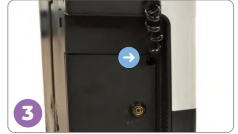
3 Position the keypad cord through the opening at the top of the Access Door. Close and re-lock the door.
