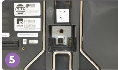
5 Unplug the power cord from the back of the ExpressVote. Pull the release latch on the cord to remove it. Next, unplug the power cord from the surge protector, and unplug the surge protector from the wall outlet.
