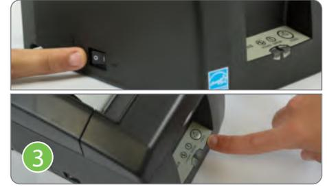
Locate the printer and its supplies. Plug the power cord into the adapter, then plug the cord into the printer. Use a surge protector to connect to power. Flip the power switch to **ON**, then press the **Feed** button for 3 seconds to test printer.
