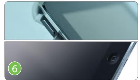
Power off the Poll Pad by holding the **Power Button** (near camera) and **Home Button** (near Lightning Connector) down until the screen turns black. Repeat steps 3-6 on every Poll Pad.
