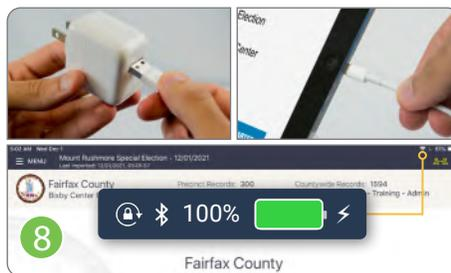
Plug the charging cable into the power cube, then plug the cable into the Lightning Connector. Use a surge protector to connect to power. Verify the battery indicator turns green and a **Charge** icon appears.
