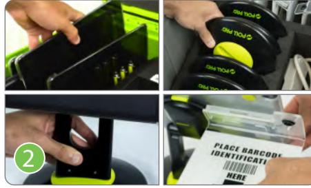
Remove the contents from the green Poll Pad Case and the gray Plastic Tote. Assemble each Poll Pad by gently inserting the Poll Pad Arm into the Base and attaching the ID Holder to the back of the Poll Pad. Do not connect to power yet.
