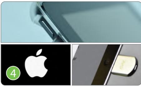
On the Poll Pad, press and hold the **Power Button** (near camera) until the Apple logo appears. After the Poll Pad powers on and the app launches, insert the iSync drive into the **Lightning Connector** (near home button).
