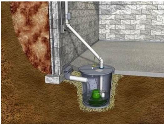
**Policy:** The sump pump discharge location must be illustrated on the grading plan when a sump pump is proposed in conjunction with the construction of a new home or substantial improvement to an existing home. The grading plan must also include the following note:
