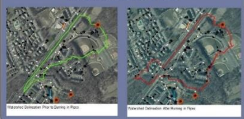
Figure 2: Results of Incorporating Stormwater Pipes into Micro Drainage Areas
