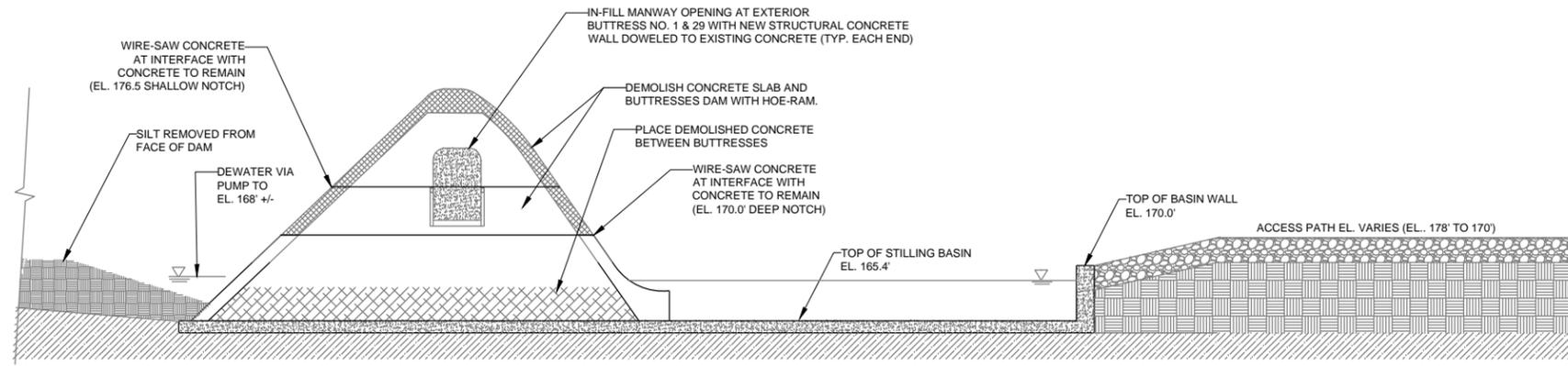
DEMOLITION - TYPICAL SPILLWAY CROSS SECTION
