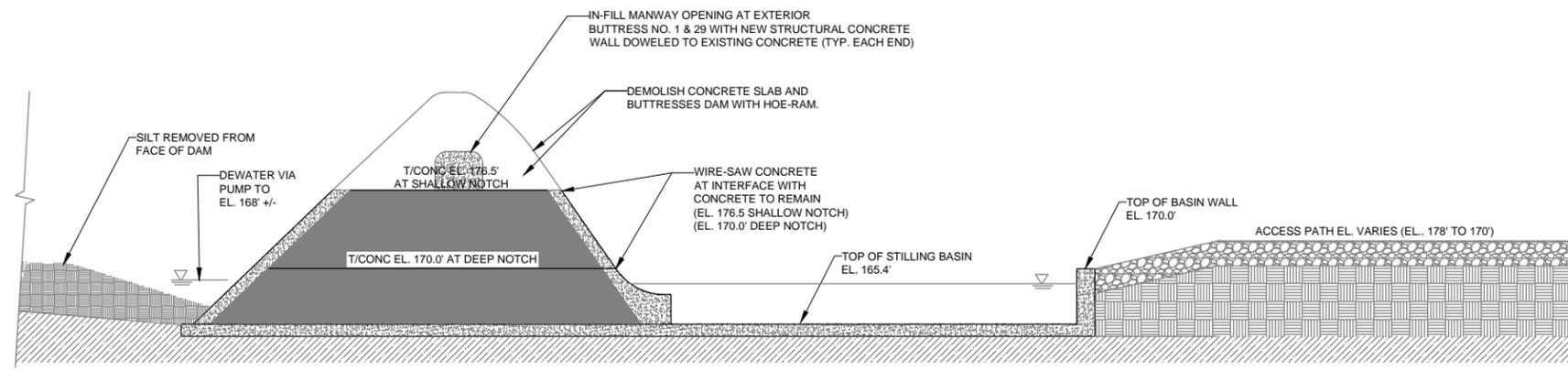
DEMOLITION - TYPICAL SPILLWAY CROSS SECTION
