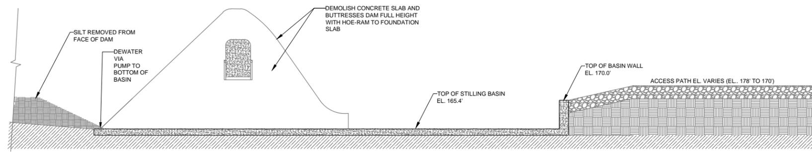
DEMOLITION - TYPICAL SPILLWAY CROSS SECTION
