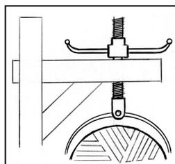
An inclined plane wrapped around a cylinder or cone.
